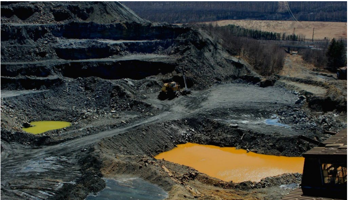
These mine pools have orange oxygenated water with high levels of iron hydroxide.
