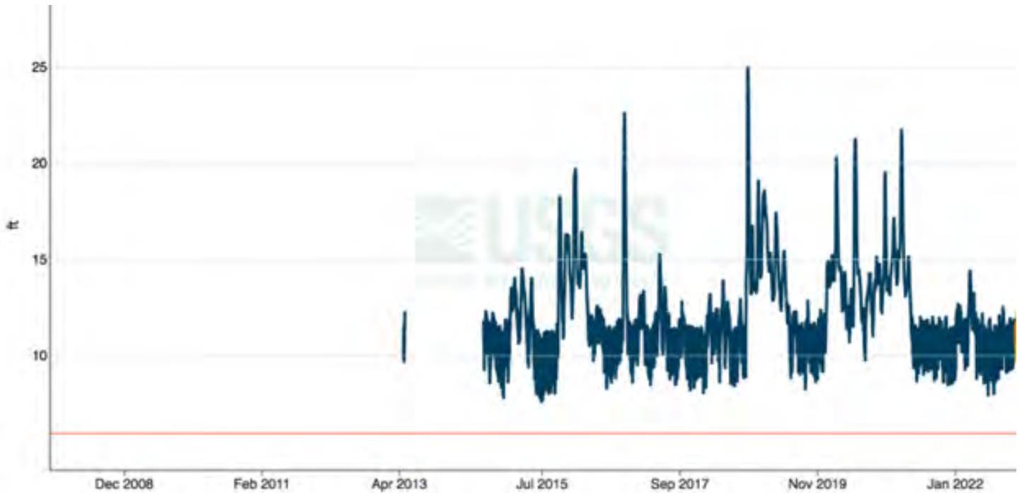
Figure 5. Hydrograph of stream gage height of Pee Dee River at Highway 701 Bucksport, South Carolina October 2007–January 2023. U.S. Geological Survey station 02135200. The red line indicates the operational limit of the monitoring station. ( https://waterdata.usgs.gov/monitoring-location/02135200 ).
